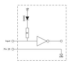
Equivalent circuit for the parallel inputs
