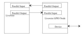
When the device triggers a status output on its parallel port, it is sent to the Livewire GPIO node's input, and is presented to the Livewire network as a Livewire GPI signal.
