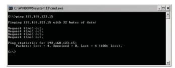
4. Much better. The time out messages indicate that no device responded at this address. This is a pretty good indication that we can use this address. But let's double check to be sure. There are some IP devices that may be configured not to reply to pings.
