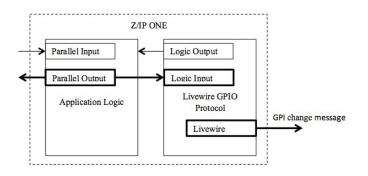
In this manner Livewire GPIO is analogous to Livewire Audio. The audio that goes out the XLR outputs is what shows up on the Livewire network as a Source. The logic signal that goes out the parallel port output is what shows up on the Livewire network as a GPI.
