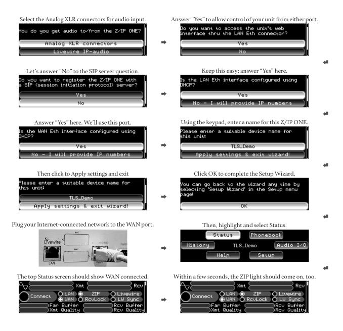
The ZIP indicator is your assurance that your Z/IP ONE is communicating with the Telos ZIP Server, and that connections to other Z/IP ONEs and Zephyr/IPs are just two button presses away.
