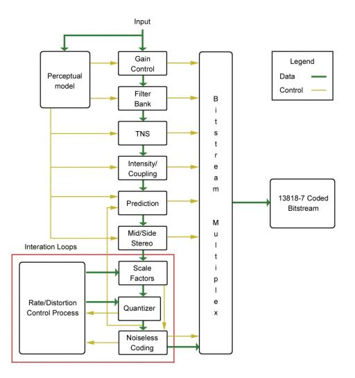
Because AAC was built on a similar structure to Layer 3, it therefore retains some of its powerful features:
