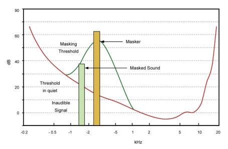
Masking effects in the frequency domain. A masking signal inhibits audibility of signals adjacent in frequency and below the threshold.
