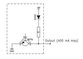
Equivalent circuit for the parallel outputs
