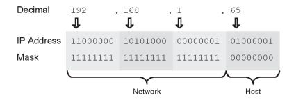
Step 3: For each 1 in the subnet mask, keep the corresponding IP address bit as is, and for each 0, convert the corresponding bit to 0. We end up with:
